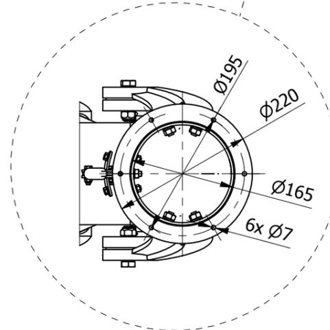
**Stainless Steel Fume Arm - Duct dia.160 mm, reach 3,0 m**
