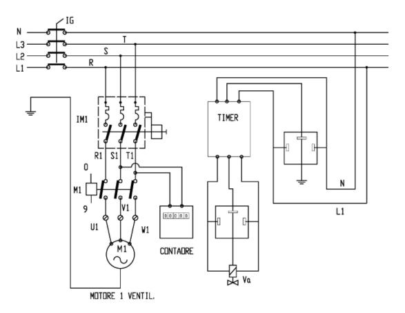
Timer and coil of the compressed air cleaning system are connected to the circuit (look scheme under section **"7.2.2. REPLACEMENT OF THE PNEUMATIC CLEANING COMPONENTS (TIMER)**").
