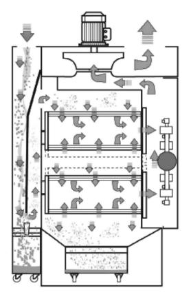
The polluted air is sucked through the air intake by the vacuum created inside the casing by the centrifugal fan.
