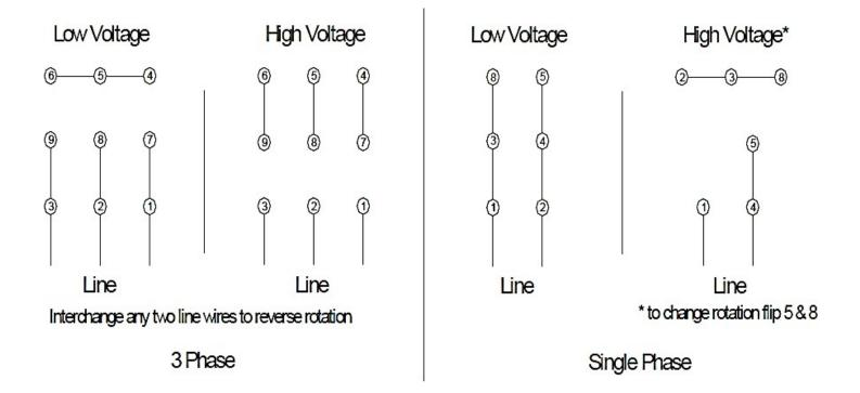
Figure 1 Wire Connection Diagram
