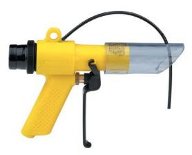
The deep hole gun is a modified version of the standard gun, designed for removing chips from blind holes. The thin black tube blasts high pressure air to dislodge chips while the main nozzle draws them safely away. A clear plastic shroud protects the operator from flying debris.
