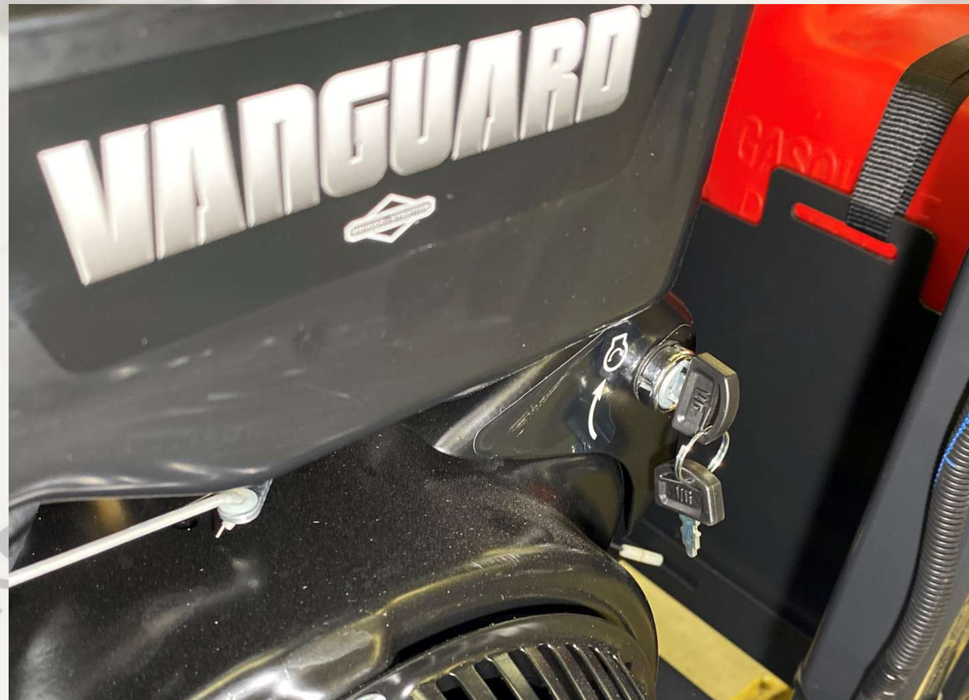
Ignition switch: rotary key switch controls ignition circuit of the machine
