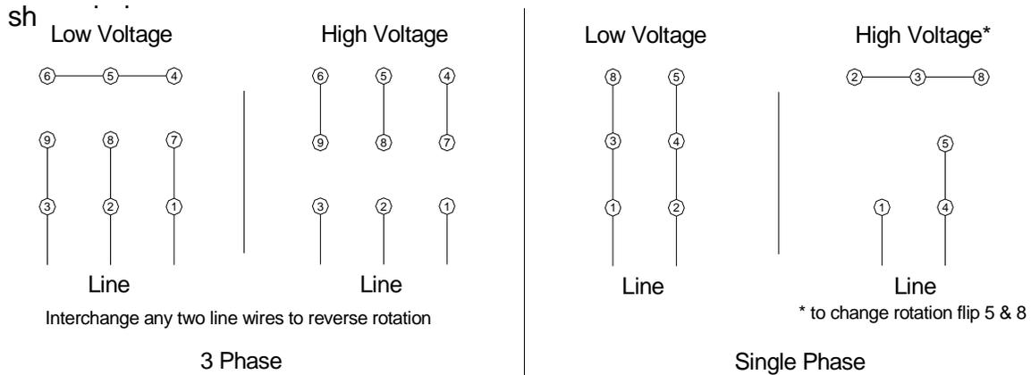
**Figure 1 - Motor Connection Diagram**
